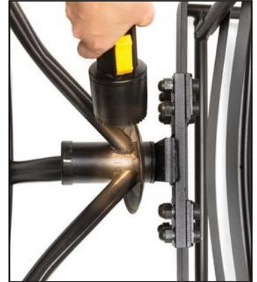
2. If the welds where each chair leg meets the center cylinder go all the way around each joint like PHOTO 1, you do not need a repair kit. If the welds where each chair leg meets the center cylinder do not go all the way around each joint like PHOTO 2, your chair is included in this recall.
